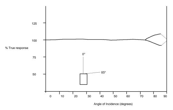
Figure 2 Typical Cosine Response Error for SP1110
