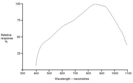
Figure 1 Typical Spectral Response of SP1110
